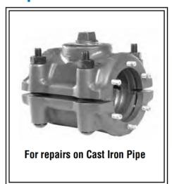
Dresser Style 80 "Ready-Pack" Split Sleeves are used to enclose and permanently repair breaks, splits and holes in cast iron pipe. Style 80 sleeves can also be used as an efficient, low-cost tapping sleeve for connecting new branch service outlets.
