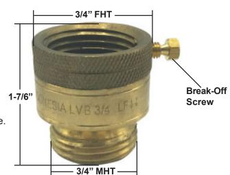
**Installation Instructions:** Screw on to hose thread of sillcock. For permanent installation: tighten break-off screw until head snaps off
