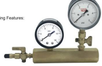
The key to the **W-R Low Pressure Gas Test Kit** is the diaphragm actuated gauge. Standard pressure gauges are <u>not</u> capable of measuring minute variations because they use a bourdon tube. This type of measuring element, which is effective for higher pressures, will not detect the minute variations in pressure when a leak exists.
