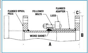
**NOTE 1:** Tie Rods are designed for 150 PSI Maximum Working Pressure. (Tie rods are optional by request)
