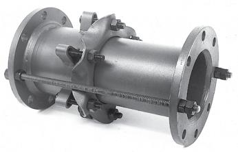
The **Dresser Dismantling Joint** is available in a variety of coatings to suit operating and environmental conditions, and gasket compounds are selected for compatibility with line content, with the standard gasket available in a Dresser Grade 27 BUNA S compound.
