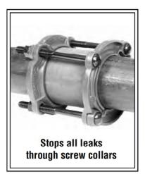
Dresser Style 4 and Style 41 Clamps quickly and inexpensively stop leaks through threaded screw collars (threaded couplings), solvent weld couplings (collars) and stab-type PVC joints. Repairs are permanent and normally made without interrupting service or dismantling the line. Style 4 clamps consists of two malleable split follower
