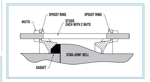
**Style 60-S Clamp for Stab-type Pipe Joints**
