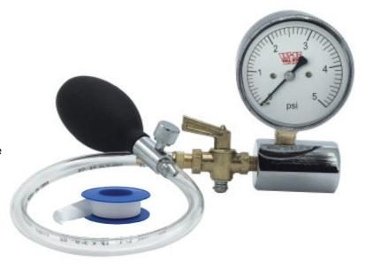
The key to the **W-R Low Pressure Gas Test Kit** is the diaphragm actuated gauge. Standard pressure gauges are <u>not</u> capable of measuring minute variations because they use a bourdon tube. This type of measuring element, which is effective for higher pressures, will not detect the minute variations in pressure when a leak exists.
